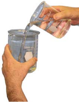
DPDM-400 High Temp Silicone Fluid remains stable at 250C (open system) & 300°C (closed system)
